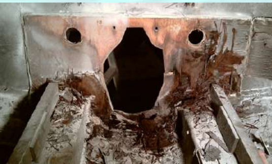
He had to rebuild the transom due to rot...
