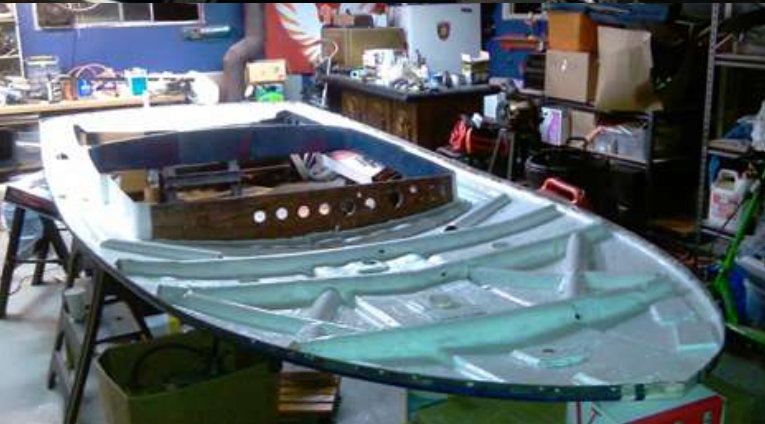
He had to rebuild the transom due to rot...
