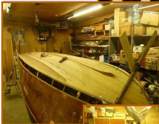
Tacking down guide prior to cutting plank.
